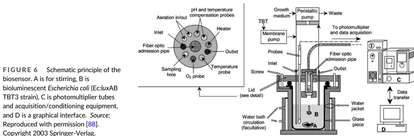
**FIGURE 6** Schematic principle of the biosensor. A is for stirring, B is bioluminescent *Escherichia coli* (*Ec:luxAB* TBT3 strain), C is photomultiplier tubes and acquisition/conditioning equipment, and D is a graphical interface. Source: Reproduced with permission [88]. Copyright 2003 Springer-Verlag.
