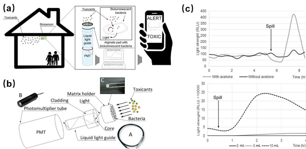
**FIGURE 5** Luminescent bacterial biosensor for real-time air quality monitoring. (a) Schematic diagram of the working principle of the biosensor, (b) structure of the biosensor, and (c) response of the biosensor in a genuine office setting to exposure to 2 mL of acetone and 5 and 10 mL of chloroform. Source: Reproduced with permission [78]. Copyright 2015 American Chemical Society.
