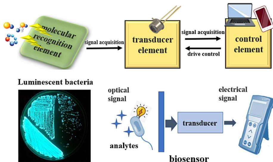
**FIGURE 1** Architecture diagram of the luminescent bacteria-based biosensor system. Luminescent bacteria reduce or stop emitting light after exposure to toxic analytes; then the transducer collects and converts optical signals into electrical signals, followed by the control element for processing the signal.
